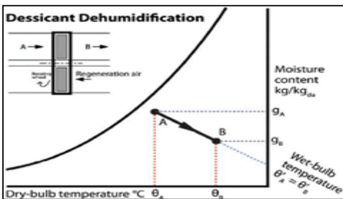
Fig.5.1: Desiccant Dehumidification Process
