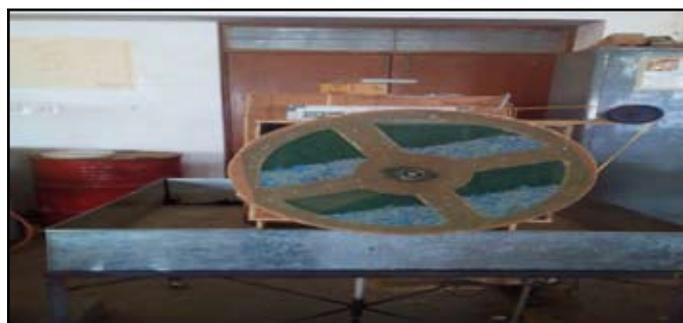
Fig. 5.3.4 : Complete Fabrication of Desiccant Wheel Dehumidifier
