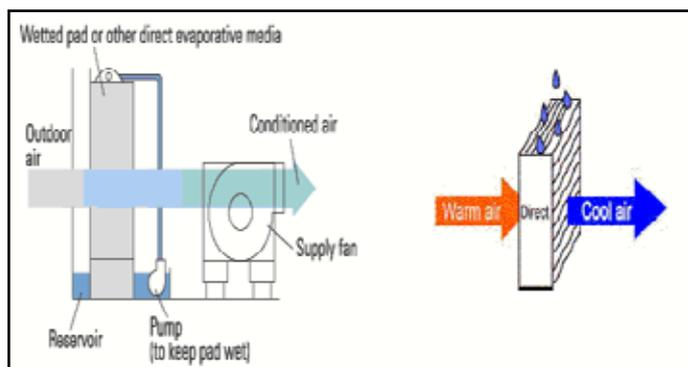
Figure 5.2 : Direct Evaporative Cooling System
