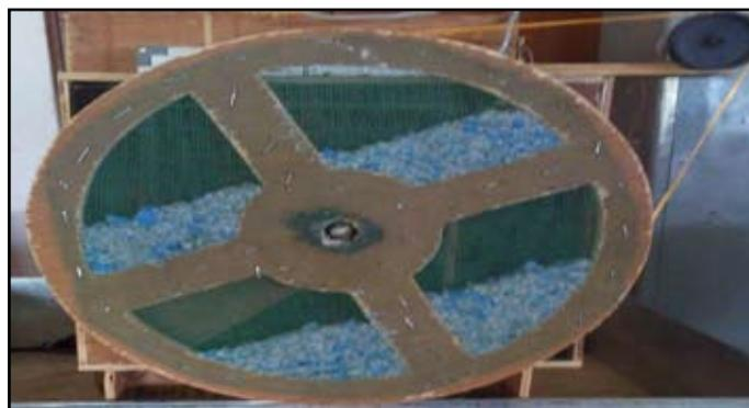
Fig. 5.3.3: Fabrication of Desiccant Wheel
