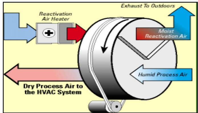
Fig. 2.5.1: Desiccant Wheel Dehumidifier
