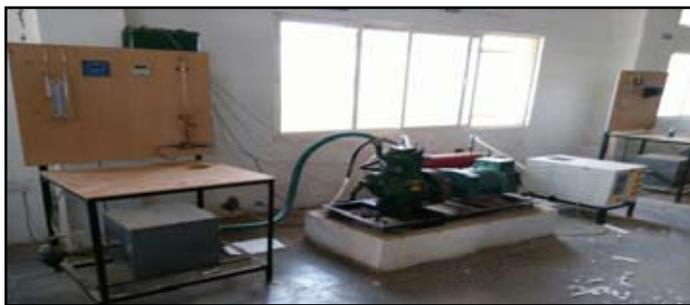
Fig.: 4-stroke diesel engine with electrical loading
