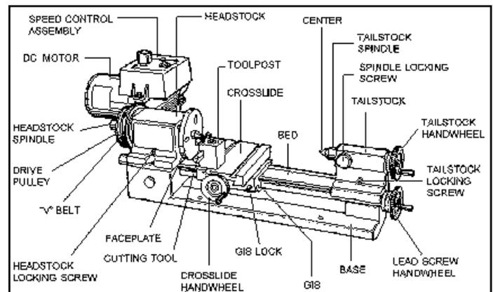
Fig. 5: Parts of Sherlin Lathe showing vertical position of various components.
