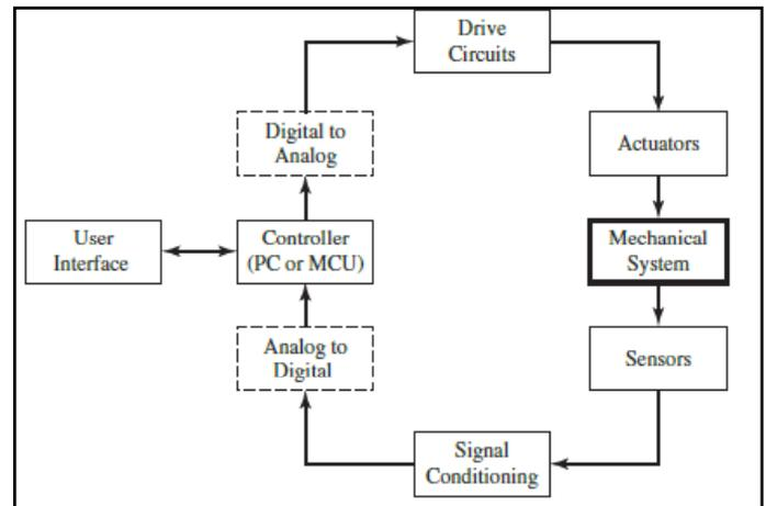
Fig. 2: Typical components of a mechatronics system
