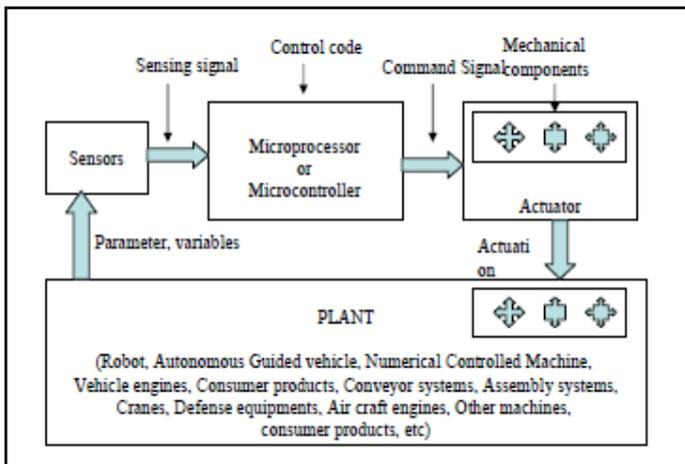
Fig.1: Schematic diagram of Mechatronics system
