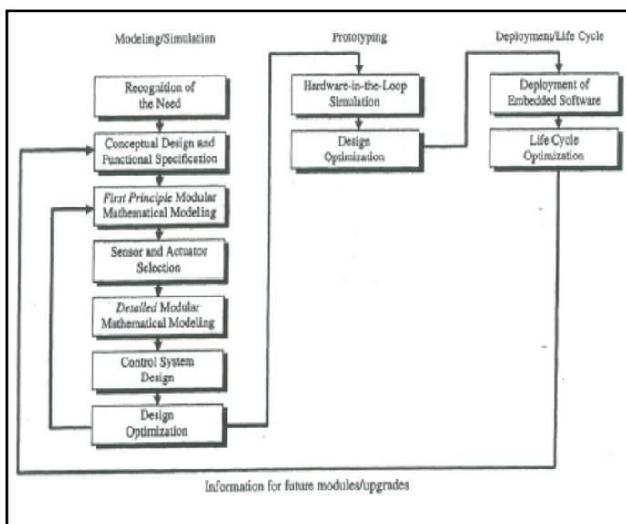
Fig. 4: The Mechatronics design process
