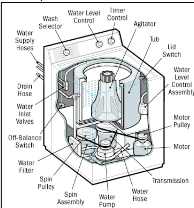
Fig. 7: Inside view of an automated washing machine
