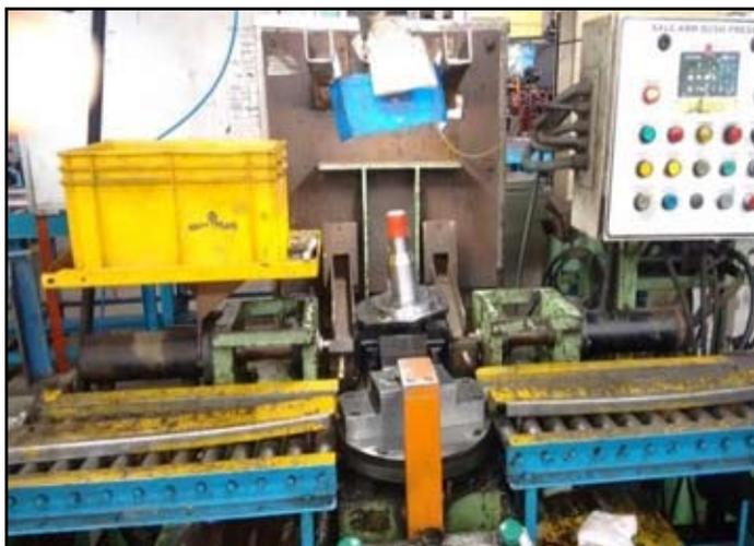
Fig 3.2. Axle bush pressing machine
