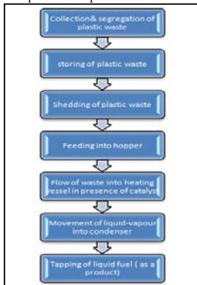
Fig No 3: Flow Chart For Steps of Production Process of Plastic Fuel
