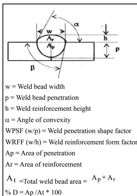
Fig.1: Bead Geometry & Shape Relationships. [3]
