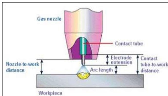
Fig. 5: Contact tube-to-work distance
