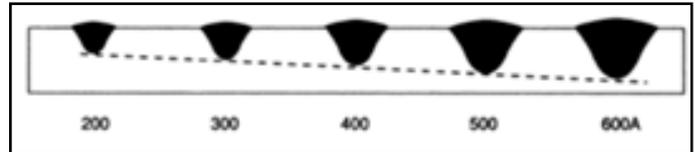
Fig. 2: Effect of Current on Weld Bead [25]
