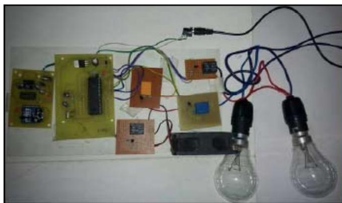
Fig. 2 : Receiver Module
