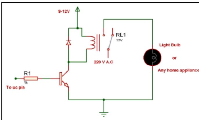
Fig. 10 : Relays switch board interfacing with the microcontroller
