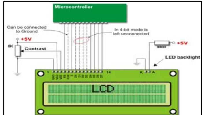
Fig. 8 : LCD Basic Connection
