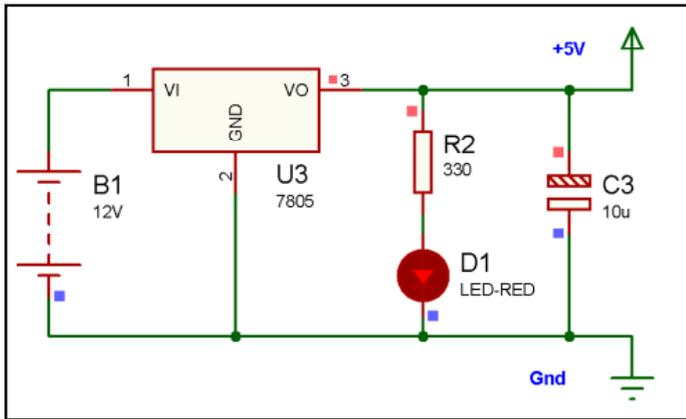
Figure 9 Battery operated +5V power supply
