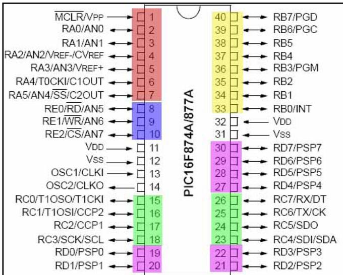
Fig.7 : PIC 16F877A Pin Configuration
