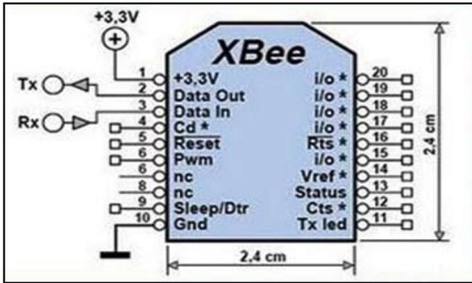
Fig. 6 : Zigbee pin configuration
