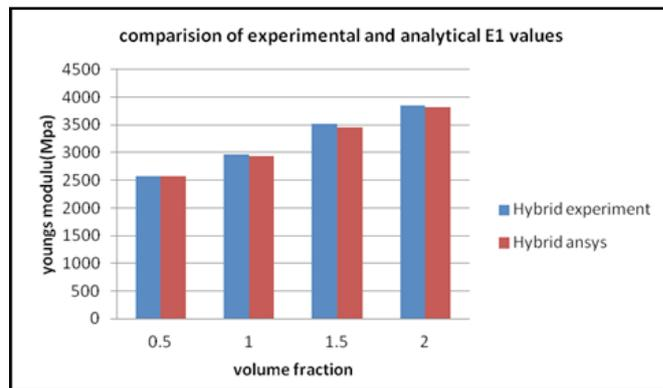
Graph 1: Comparison plot of tensile modulus for different fiber configurations.
