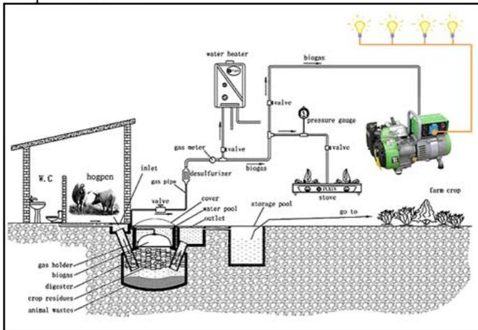
Fig: Schematic of a biogas plant used for power generation
